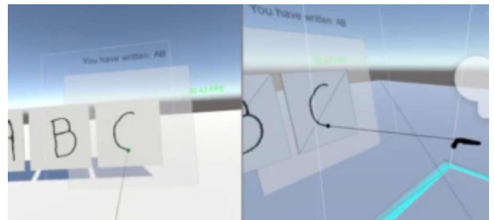
Figure 2 Experimental implementation of handwriting recognition input in VR (Elmgren, 2017)
